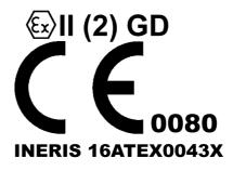
Single marking complies with all of applications covered by the ATEX certification of the drive.
