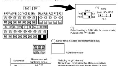
(Blade thickness: 0.5 mm, blade width: 3.5 mm)
