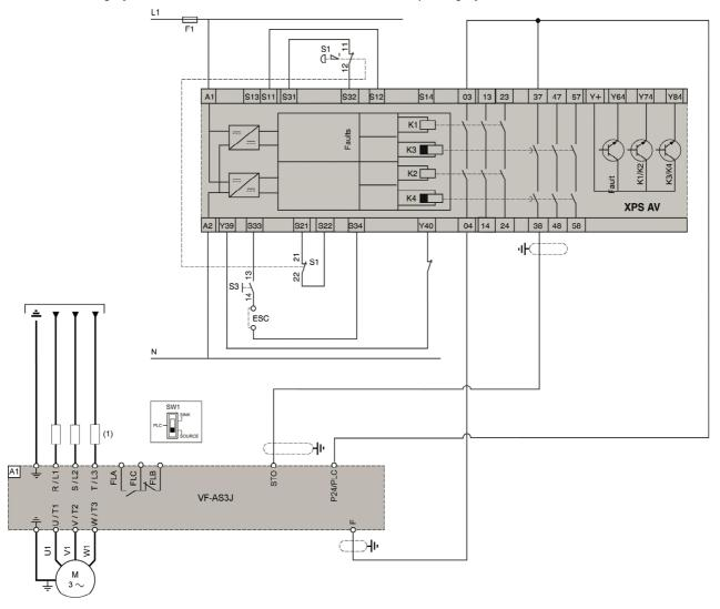
**NOTE:** This diagram is a wiring configuration using F assigned to forward operation.
