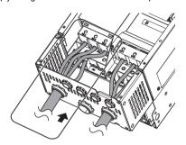
10 When connection is complete, mount the front cover. For how to mount, refer to [2. 2. 2].
