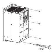
2 Lift the front cover and remove it from the unit.
