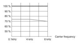
40°C(104°F) - Standard installation, Side-by-side installation, with NEMA Type 1 kit
