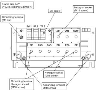
The wire strip length is 32 mm and the tightening torque depend on wire size. Refer to [4. 1 Selection of wire size].
