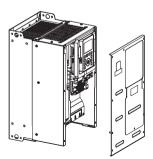
3 Mount the front cover in the reverse procedure. Tighten the screws to 1.5 N·m / 13.2 lb·in.
