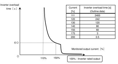
Inverter overload protection characteristic
