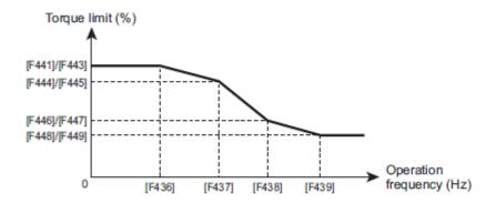
Set four points, (F436, F441/F443), (F437, F444/F445), (F438, F446/F447), and (F439, F448/F449). You can change the torque limit level with the run frequency.
