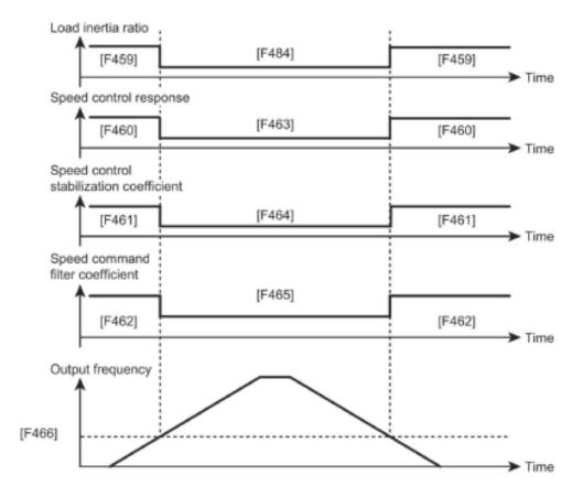
In a range where the output frequency is [F466] or less, [F460], [F461], and [F462] are enabled. In a range where the output frequency is over [F466], [F463], [F464], and [F465] are enabled.
