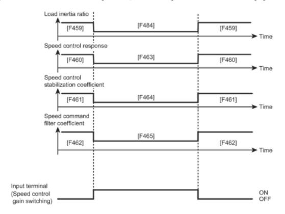
By using [F466] together with the speed gain switching by the input terminal, you can switch between speed control gain 1 and speed control gain 2.
